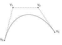
In general, the *n*th derivative at an endpoint depends only on the n+1 points nearest that endpoint.
