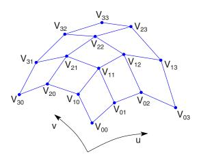
Given a grid of control points  $V_{ij}$ , forming a **control net**, contruct a surface S(u,v) by:
