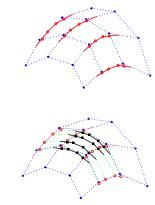
Which B-spline control points are interpolated by the surface?
