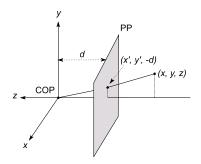
By similar triangles, we can compute how much the *x* and *y* coordinates are scaled:
