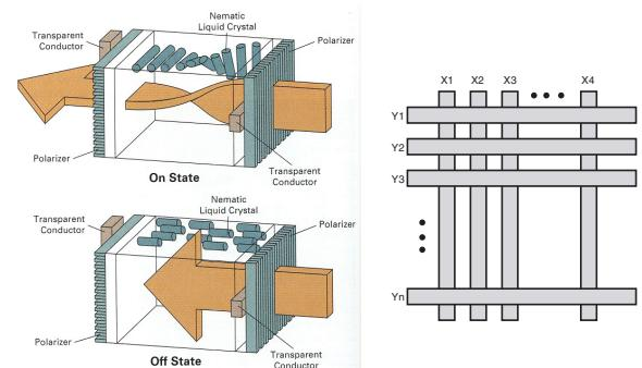
Laptops typically use **liquid crystal displays (LCD's)**.
