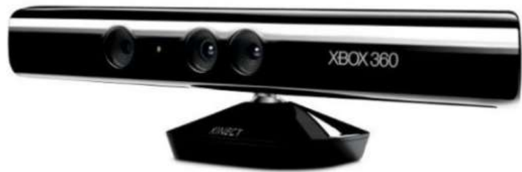
Structured light projection
