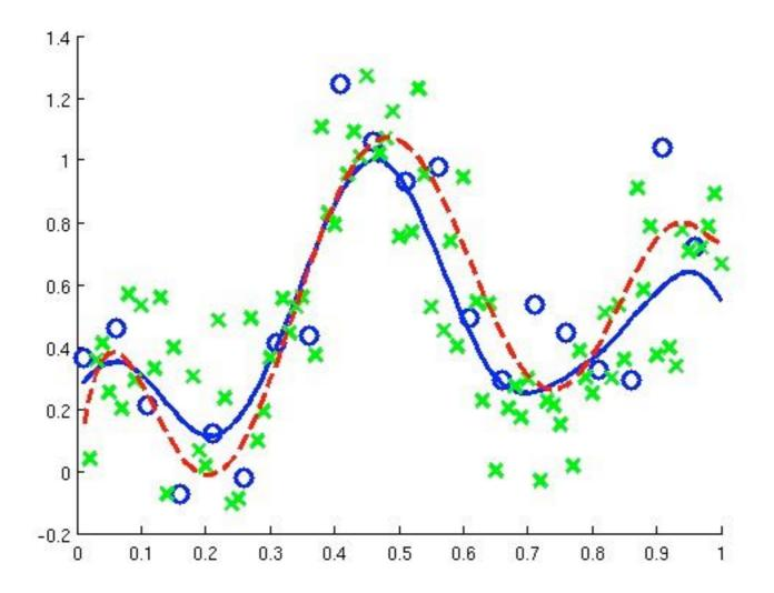
• Calculate rms error  $e_{rms} = \left(\frac{1}{N}\sum_{i}(y_i - \hat{y}_i)^2\right)^{\frac{1}{2}}$
