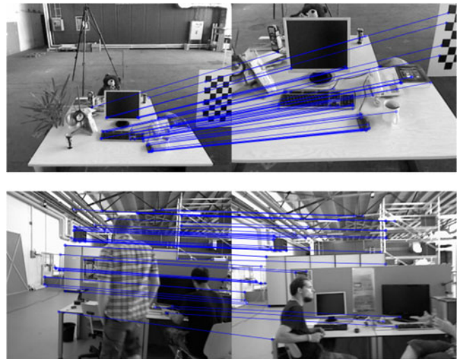
Fig. 8. Example of challenging relocalizations (severe scale change, dynamic objects) that our system successfully found in the relocalization experiments.
