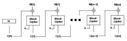
Figure 2 - CBC Encryption Algorithm
