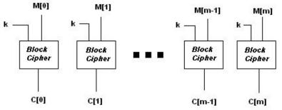
Figure 1 – Electronic Code Book (ECB) mode encryption algorithm
