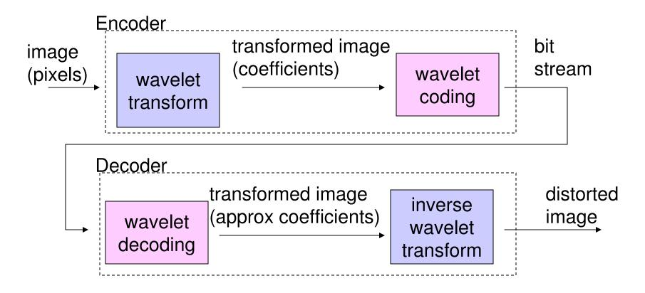
Wavelet coder transmits wavelet transformed image in bit plane order with the most significant bits first.
