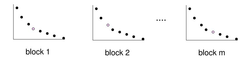
Pick one point from each curve so that the sum of the x values is bounded by R and the sum of the y values is minimized.
