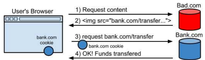
Figure 2: An example CSRF attack. When the user visits the adversary’s page, the HTTP reply (step 2) includes code that causes the user’s browser to make a request to bank.com (and attach bank.com ’s cookie). Bank.com erroneously treats this request as legitimate since it has the user’s cookie.
