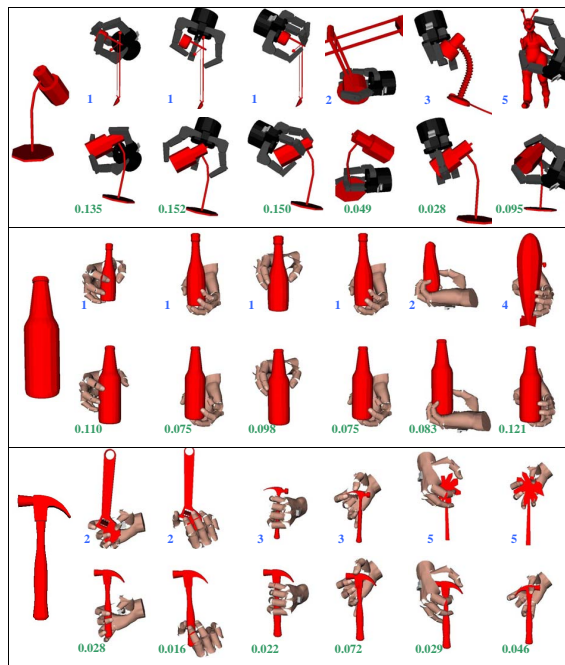
Figure 1: Three example models and their grasps from neighbors in the grasp database
