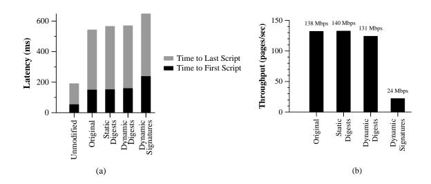
Figure 7.7: Performance impact of whitelists. (a) Impact on client perceived latency. (b) Impact on server throughput. In both graphs, the four pages use no whitelist, a static whitelist, a whitelist of digests generated on the fly, and a whitelist of signatures generated on the fly, respectively. For client latency, we also show the performance of an unmodified browser on the original page.
