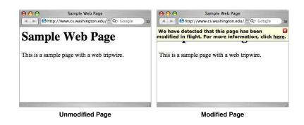
Figure 6.2: If a web tripwire detects a change, it displays a message to the user, as in the screenshot on the right.
