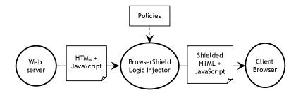
Figure 8.1: BrowserShield transforms HTML and JavaScript into safe equivalents, using a set of policies as input.
