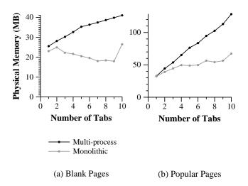
Figure 5.4: Memory overhead for loading additional blank or realistic pages in new tabs.
