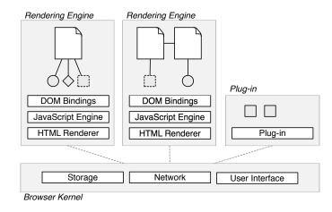
Figure 5.1: A multiprocess architecture can isolate web program instances and their supporting browser components, from each other and from the rest of the browser. Plug-ins can also be isolated from the rest of the browser. Gray boxes indicate processes.
