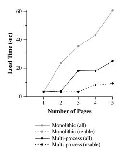
Figure 5.2: Solid lines show the total load time for restoring a session of realistic pages. Dotted lines show the time until at least one of the restored pages is usable. Both lines for the monolithic architecture overlap.
