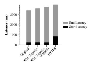
Figure 6.3: Impact of web tripwires and HTTPS on client perceived latency.
