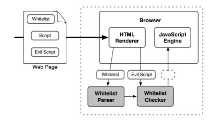
Figure 7.5: Architecture of enhanced browser prototype. The parsing logic delivers each page's whitelist to an external checking mechanism. The browser then consults the checking mechanism before giving each script to its JavaScript engine.
