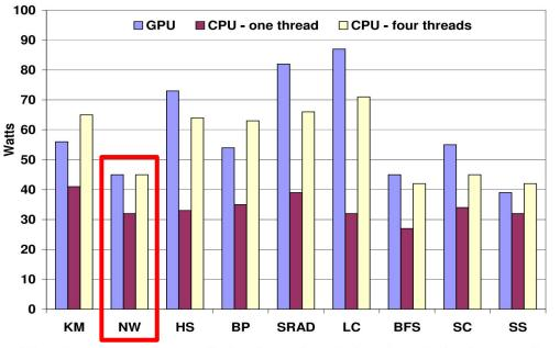
Fig. 5. Extra power dissipation of each benchmark implementation in comparison to the system's idle power (186 W).
