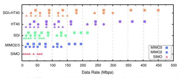
Figure 3.1: The different rate-related 802.11n configurations that use three antennas and 802.11n physical layer enhancements.
