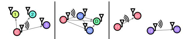
Figure 1.3: The three key configuration problems in multi-device networks. *Left:* access point selection. *Center:* Multi-hop mesh routing. *Right:* Spatial reuse.
