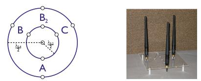
Figure 5.2: The antenna stand I use to achieve consistent spatial geometry for desktop machines. It supports circular and linear arrays of two or three antennas with the correct  $\lambda/2$  separation at either 2.4 GHz or 5 GHz.
