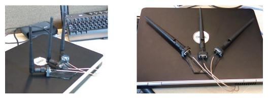
Figure 5.3: One of the three laptops, pictured here, includes a custom antenna mount for a 2.4 GHz linear array.
