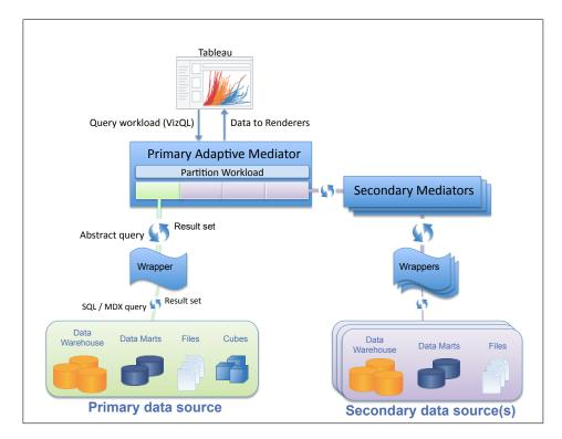
Figure 2.3: Tableau's data blending architecture
