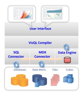
Figure 2.1: Architecture of Tableau
