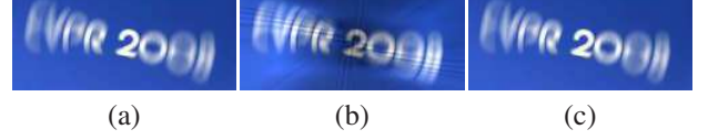
Figure 4. Convolution with kernel decomposition. (a) Convolution result without kernel decomposition, where full-sized kernels are generated on-the-fly per-pixel. (b) Convolution using 30 PCA-decomposed kernels. (c) Convolution using delta function decomposition of kernels, with at most 30 delta functions per pixel.
