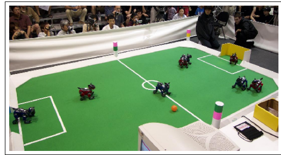
Fig. 1. Legged AIBO robots during a RoboCup match. Color information is extremely important since all robots have the same shape and the outline of the environment is completely symmetric.
