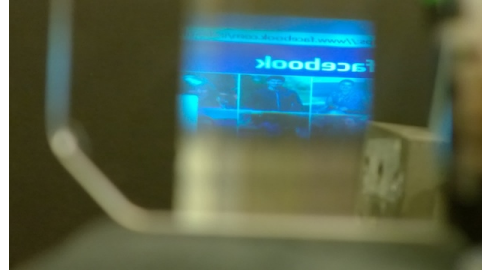
Figure 5: Display leakage from the Lumus. The image is clear and visible from a distance, but only a small portion is visible from each vantage point.
