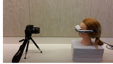
Figure 3: Experimental setup for evaluating the display leakage of the Silicon Micro Display ST-1080.
