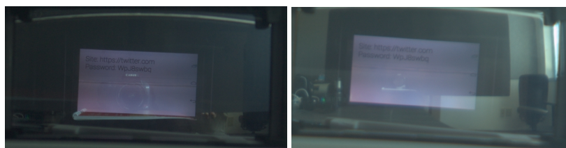
Figure 17: Images of the Silicon Micro Display, displaying a black on white password manager screen, from 0.35m and 1.4m away. The reader may wish to experiment by zooming into these images in the PDF.
