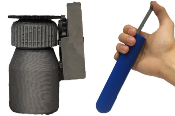
Figure 14: Application prototypes. (a) shows our pill bottle prototype and (b) shows our insulin pen case. For the latter, the user pushes the plunger to use the insulin pen, which in turn uses our ratchet mechanism to store the usage data.
