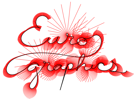
Figure 1: A clothoid spline sketched using our algorithm. The red comb illustrates curvature along the path.
