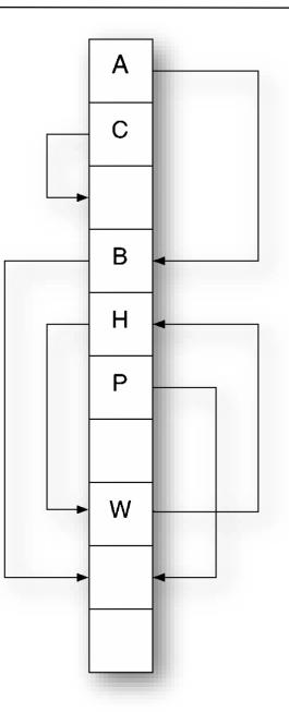
Alternately (as in the picture), we can use a single table with 2M entries and two hash functions  $h_1, h_2: \mathcal{U} \rightarrow [2M]$  (with the same "bumping" algorithm)
