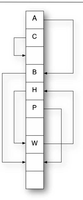
**Data structure:** Two tables  $A_1$  and  $A_2$  both of size M = O(N)Two hash functions  $h_1, h_2 : \mathcal{U} \to [M]$ (will assume hash functions are fully random)
