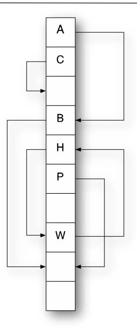
**Data structure:** Two tables  $A_1$  and  $A_2$  both of size M = O(N)Two hash functions  $h_1, h_2 : \mathcal{U} \to [M]$ (will assume hash functions are fully random)
