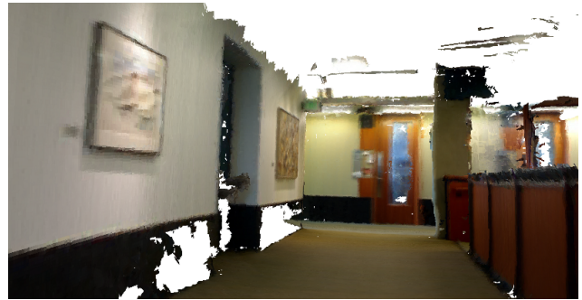
Figure 1: Model built with our method at a resolution of 2 cm. The surface is represented with surface patches of size 20\text{ cm} \times 20\text{ cm} . Each patch is encoded with a sparse code of an overcomplete dictionary. Generated from a 3.35 GB dataset, the resulting file size is 10.2 MB.
