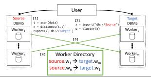
**Figure 2.** Using the data pipe generated by PipeGen for the hybrid analysis from Section 2: 1. User submits a query to the source DBMS (e.g., Myria) to compute distance and export to the target DBMS using data pipe. 2. User issues an import query on the target DBMS (e.g., Spark) to cluster the result. Data is transferred using the generated data pipe in 3., and in 4. a worker directory (see Section 4.3) coordinates the connection process. PipeGen-related components are highlighted in green.
