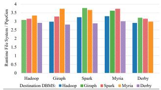
**Figure 9.** Total speedup between file system and PipeGen for 10<sup>9</sup> elements. Transfer occurred from a source DBMS (*x*-axis) to a destination DBMS (bar color/pattern) using CSV. The number of workers/tasks was fixed at 16.
