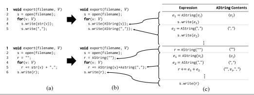
**Figure 8.** (a) Two ways to implement CSV export (inserting newlines instead of a comma on the last value is omitted for clarity); (b) after replacement of literals and conversions; (c) accumulated values in AString instances after one iteration.
