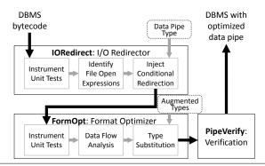
**Figure 3.** Compile-time components of PipeGen. The file IO redirector (IORedirect) generates a data pipe to transfer data via a socket, while the format optimizer (FormOpt) improves efficiency for text-oriented formats.
