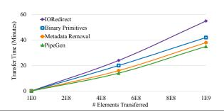
**Figure 12.** Runtime of a transfer from Spark to Giraph using the library extension mode for the Jackson JSON library. We show a baseline application of only IORedirect. We then transmit fixed-width values in binary form. Next, we remove repeated column names and delimiters. The PipeGen series shows these optimizations plus column pivoting (i.e., all optimizations).
