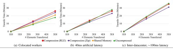
**Figure 15.** Transfer time between Myria and Giraph using compression. We show transfer for (a) workers on the same physical node, (b) 40ms artificially-introduced latency, and (c) separate datacenters (approximately 100ms latency). For RLE, zip, and uncompressed formats we transfer data over a socket. For colocation we also show transfer using uncompressed shared memory.
