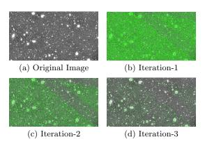
Figure 5: Snapshots from the first 3 iterations of the "sigma-clipping" algorithm with incremental optimization on the LSST dataset. Green-colored points are the ones that change across iterations. As the iterative computation proceeds, the number of green-colored points drops dramatically.
