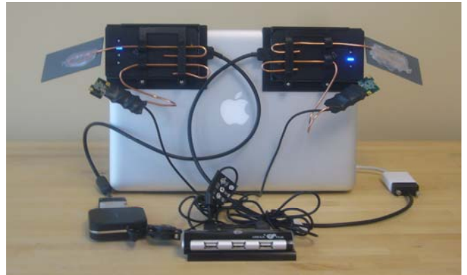
Figure 2. Rear view of the Bonfire prototype hardware setup. Projectors and cameras are mounted on the laptop screen and connected via a USB hub. Mirrors reflect the projected images to the sides of the keyboard.
