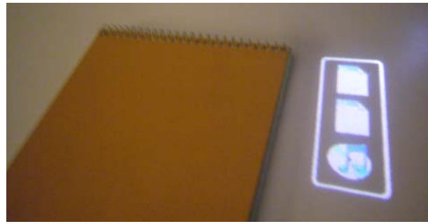
Figure 6. Physical bookmarks for digital tasks. When the notebook is detected on the table, Bonfire projects a list of applications that were open when the notebook was last seen.
