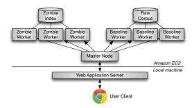
Figure 2: The IDE's basic runtime architecture.
