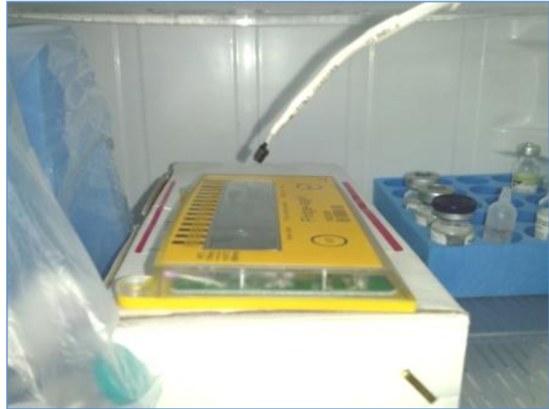
Interior view showing sensor, FridgeTag and vaccines
