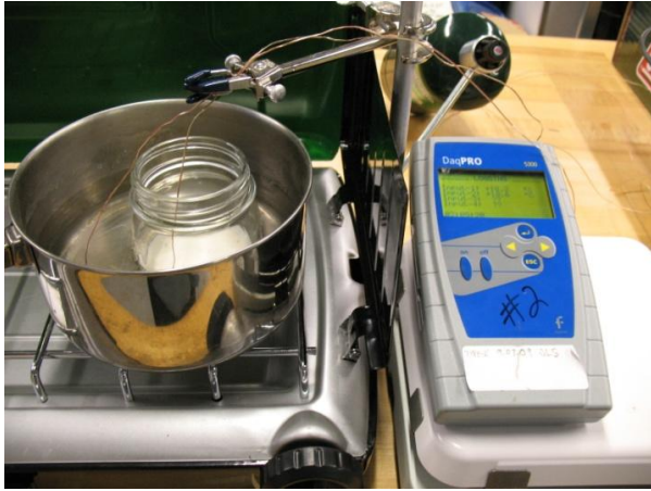
Figure 6: Experimental setup. A glass jar with milk in it is placed in a water bath and heated on a stove. Two thermocouple probes connected to a DaqPRO data logger are used to monitor the temperature of milk and water respectively.
