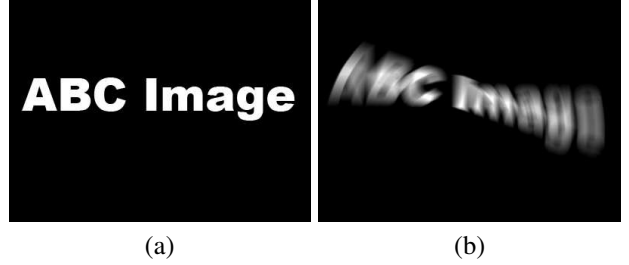
Figure 3. Rotational blur image synthesis. (a) The original image. (b) The blurred image generated using DFT. The naturalness validates the correctness of our motion descriptor.
