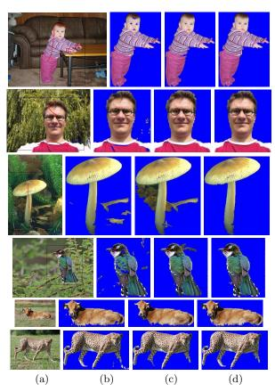
Figure 3: Comparisons between the graph-cuts over regions (GCR), the MSRM method [16] and the proposed algorithm. (a) The source images with user input stokes, where blue strokes are used to mark the background regions, and red strokes are used to mark the foreground regions. (b) Results obtained by the GCR method. (c) Results obtained by the MSRM method. (d) Results obtained by the proposed algorithm.
