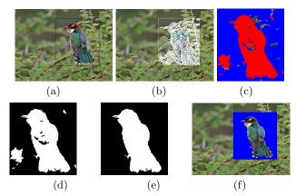
Figure 2: Steps of the proposed algorithm: (a) Original image with user input. (b) Over-segmentation by the mean-shift algorithm. (c) Result after disciminative clustering, with red indicating foreground, blue indicating background, and original color indicating ambiguous regions. (d) Result after merging ambiguous regions from (c). (e) Result of local neighborhood pruning. (f) Final result on color image with bounding box shown.
