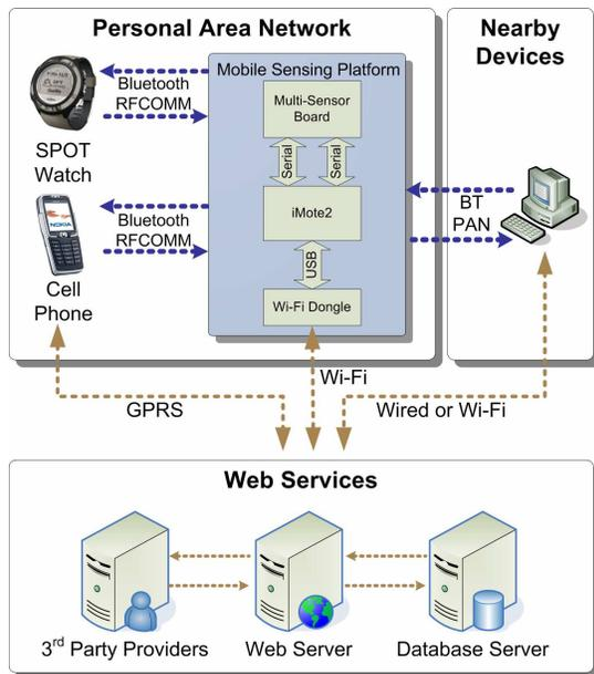
Figure 7. System Architecture
