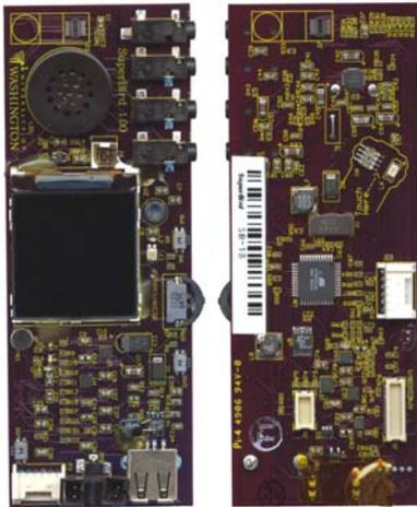
**Figure 3.** The top and bottom of the Intel iMote2 “SuperBird” board containing LCD, microphone, speaker, jog dial (near center), USB connector (left, on bottom right), and heart rate sensor (diagonally arranged area on right).
