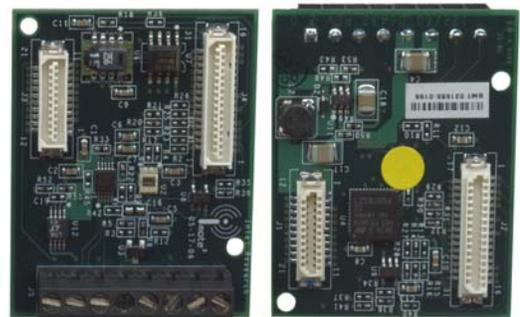
**Figure 2. The top and bottom of the Intel iMote2 basic sensor board. The 3-D accelerometer sensor is just below the yellow dot on the right.**
