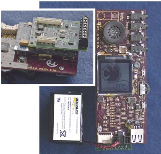
**Figure 4.** The three-board set stacked together with their rechargeable battery. The side view in the inset on the left shows the other two boards that lie below the large board in the larger picture.
