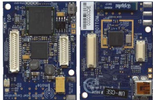
**Figure 1. The top and bottom of the Intel iMote2. The top, on the left, has the PXA271 and memory in the large chip at the top center. The bottom, on the right, has the 802.15.4 ChipCon2420 radio (within the square in the center). The long connectors on both sides connect to the other two boards.**
