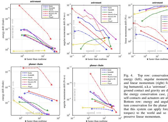
Top row: conservation of kinetic energy (left), angular momentum (center) and linear momentum (right) for the floating humanoid, a.k.a 'astronaut'. In all cases ground contact and gravity are disabled. For the energy conservation case, joint limits, self-contacts and actuators are also disabled. Bottom row: energy and angular momentum conservation for the planar chain. Note that this system can apply forces (but not torques) to the world and so it does not preserve linear momentum.
