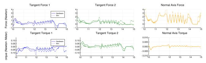
Fig. 3. In these plots, we seed our simulator with the state measured from the hardware system. We use the simulator to calculate the instantaneous forces measured by a simulated force sensor, per time-step of real world data, and compare it to the data collected from hardware. These plots are in the frame of the contact, with the force along the normal axis being greatest. Note that the Y-axis of the Normal Axis Torque plot is different from the other torque plots.
