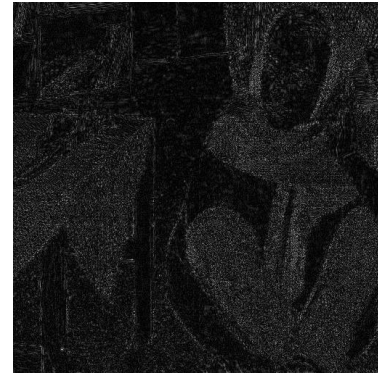
(b) JPEG2000 Rate 0.075; Compression 13.3:1 ; PSNR = 31.98 dB
