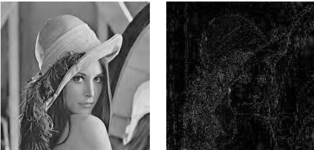
Figure 4.16: Lena after quantizing 20000 coefficients with step size 100; PSNR = 33.08 dB
