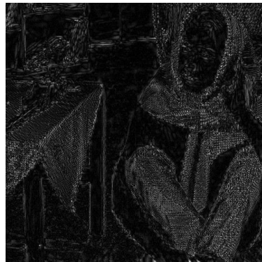
(c) JPEG2000 Rate 0.02; Compression 50:1 ; PSNR = 25.44 dB
