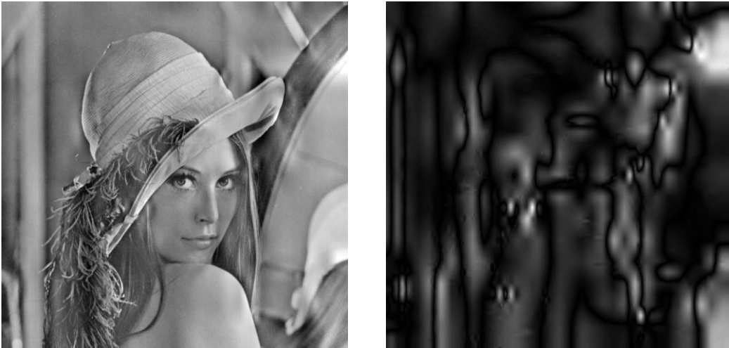
Figure 4.13: Lena after zeroing 100 coefficients; PSNR = 20.39 dB
