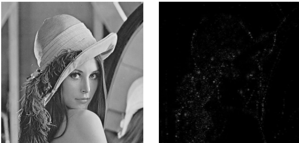
Figure 3.67: Lena: decomposition 2, tree 150000, coefficient skipping
