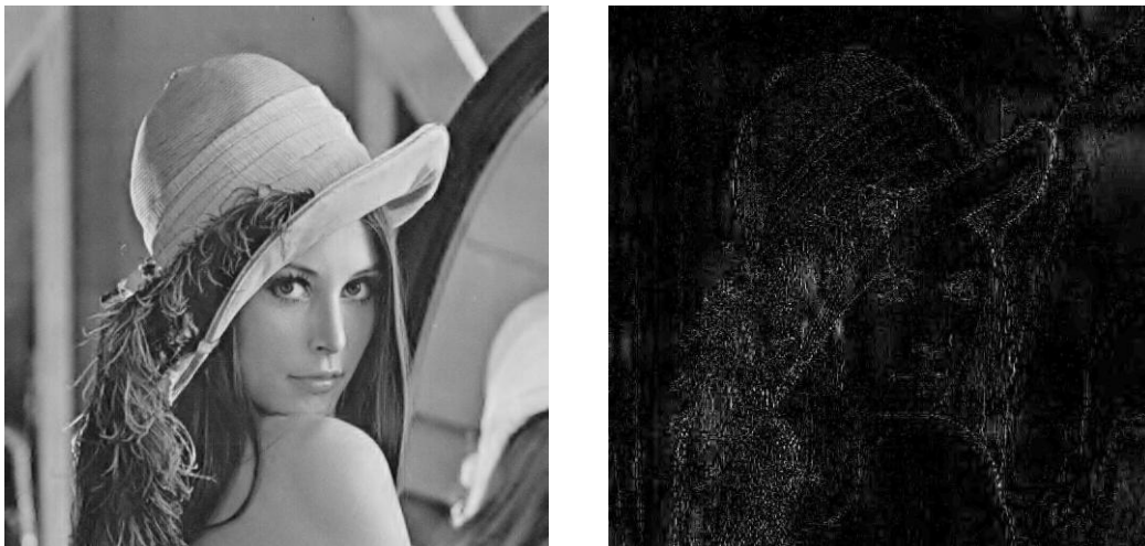
Figure 4.18: Lena after perceptually quantizing 20000 coefficients; PSNR = 35.45 dB
