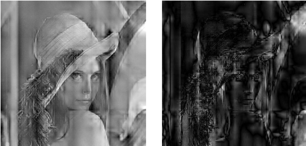
Figure 4.15: Lena after zeroing 20000 coefficients; PSNR = 19.41 dB
