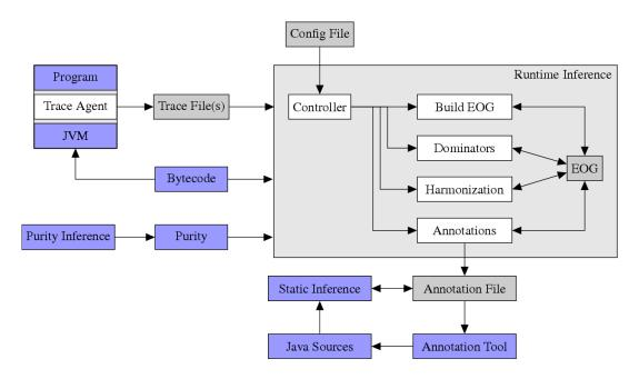
Figure 6: Architecture of the runtime inference tools. White boxes depict components of the inference tool. Boxes in light gray depict files and data structures that are part of the inference tool, and boxes in dark gray depict external components and files.
