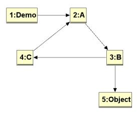
Figure 2: The store at the end of method main in class Demo. Objects are depicted by rectangles and are labeled with an identifier and the class name. References are depicted by arrows.
