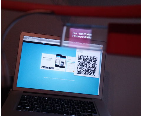
Figure 6: Prototype AR Password Manager. Our Chrome extension (background) displays a QR code representing the current website. In response to the voice command “find password,” our Google Glass application (foreground) scans this QR code and displays the stored password for that site privately in the heads-up display.
