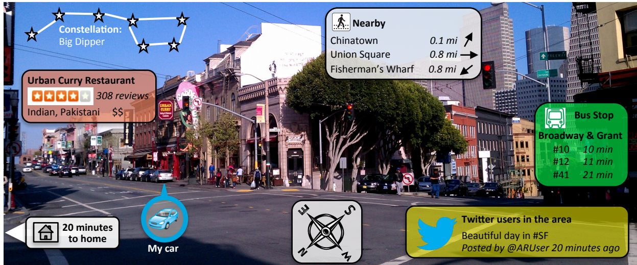
Figure 4: Multi-Application Augmented Reality. Emerging and future augmented reality platforms will support multiple applications running simultaneously, sharing input and output devices, and exposing data and APIs to each other. In a multi-application AR system, applications like those depicted in this mockup will share output devices, including displays, audio output, and haptic feedback. Conflicts among these applications can result in security concerns (Section 2.2).
