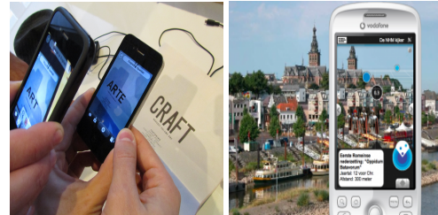
Figure 1: Phone-Based Augmented Reality. On the left, a picture of Word Lens, an iPhone application that provides seamless “in-picture” translation (source: http://www.flickr.com/photos/neven/5269418871/ ). Here the app translates the word “Craft” from English to Spanish and then back again. On the right, a picture of Layar, an “augmented reality browser” shipping on Android phones (source: http://site.layar.com/company/blog/make-your-own-layar-screen-shot-with-the-dreamcatcher/ ).
