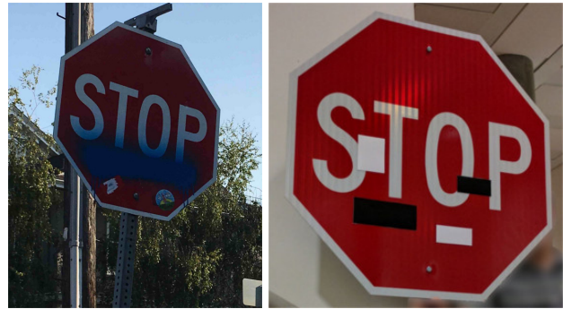
Figure 3.1: The left image shows real graffiti on a Stop sign, something that most humans would not think is suspicious. The right image shows our a physical perturbation applied to a Stop sign. We design our perturbations to mimic graffiti, and thus “hide in the human psyche.”
