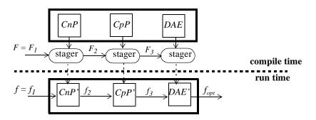
FIGURE 3.11: Staging a Three-Phase Compiler Pipeline.
