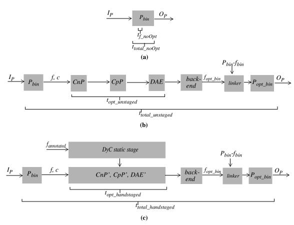
FIGURE 8.2: Baseline Configurations for Evaluating SCF. (a) Single stage, no dynamic compilation (b) Single stage, all dynamic (c) Two stages, hand-staged dynamic compilation
