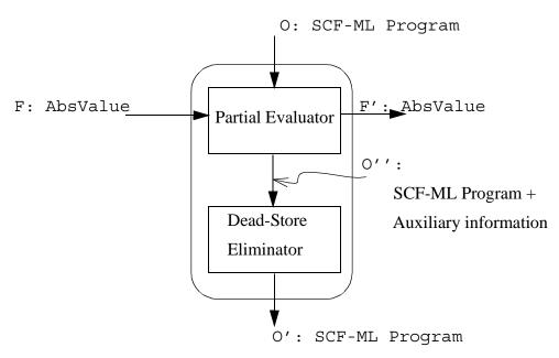
FIGURE 3.15: Internal Structure of the Stager.
