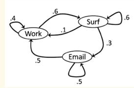
$$\begin{bmatrix} q_W^{(t)}, q_S^{(t)}, q_E^{(t)} \end{bmatrix} \begin{bmatrix} 0.4 & 0.6 & 0 \\ 0.1 & 0.6 & 0.3 \\ 0.5 & 0 & 0.5 \end{bmatrix} = \begin{bmatrix} q_W^{(t+1)}, q_S^{(t+1)}, q_E^{(t+1)} \end{bmatrix}$$
