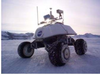
Nomad robot searches for meteorites in Antarctica http://www.frc.fi.cmu.edu/projects/meteorobot/index.html
