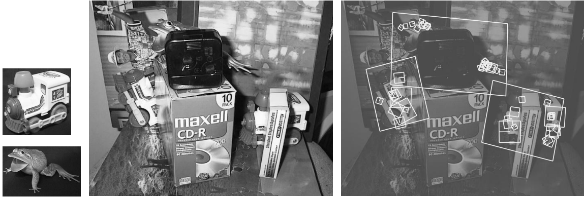
Figure 12: The training images for two objects are shown on the left. These can be recognized in a cluttered image with extensive occlusion, shown in the middle. The results of recognition are shown on the right overlaid on a reduced contrast version of the image. A parallelogram is drawn around each recognized object showing the boundaries of the original training image under the affine transformation solved for during recognition. Smaller squares indicate the keypoints that were used for recognition.
