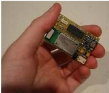
Figure 3: Wireless accelerometer board
