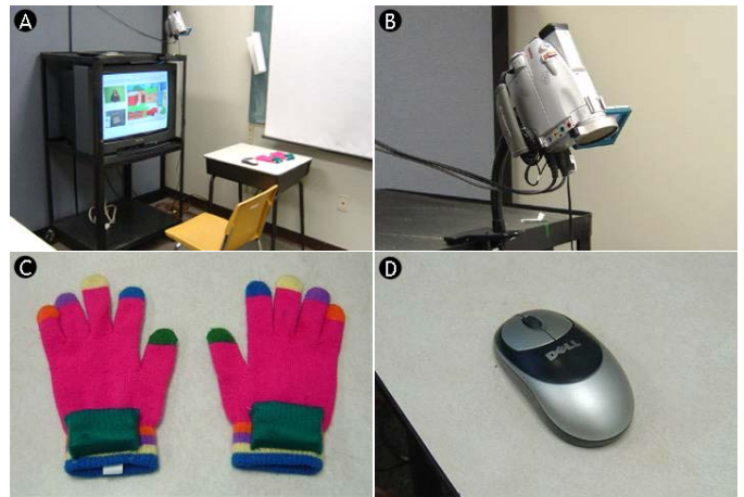
Figure 2: System setup. a) the workspace b) IEEE1394 camera c) colored gloves with wireless accelerometers in green-colored pockets d) wireless mouse
