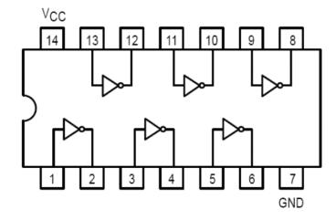
The best way is to look at the chip maps to determine the orientation and chip inputs and outputs for any of the chips we have provided for you. This '04 Chip has 6 inverters in one package - pick one of them to use. Hook up a slider switch to the inverter's input, and an LEDR to the inverter's output. Now turn on the power and flip the switch a few times – does it work correctly?
