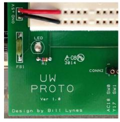
There is a fuse (FS1) and an indicator light (the blue LED) on your prototyping board. If you do accidentally wire up GND to VDD, you will mostly likely blow the fuse "F1" and the LED light will go off.
