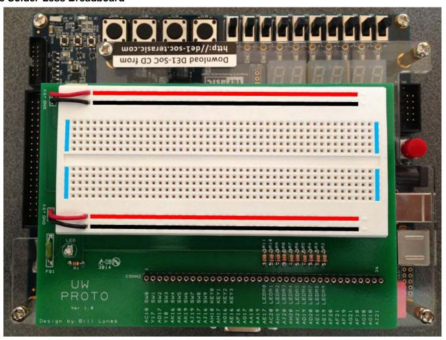
The white solder-less breadboard attached to your DE1 is where you will be building your first few circuits. Notice the red and black wires going to each of the rows at the top and bottom of
