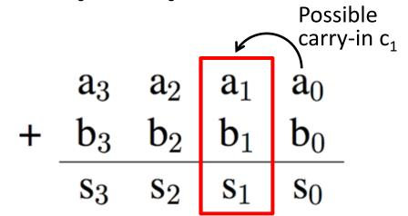
$$\begin{aligned} \boldsymbol{s_i} &= \mathrm{XOR}(a_i, b_i, c_i) \\ \boldsymbol{c_{i+1}} &= \mathrm{MAJ}(a_i, b_i, c_i) \\ &= a_i b_i + a_i c_i + b_i c_i \end{aligned}$$
