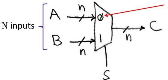
This input is passed to output if selector bits match shown value
