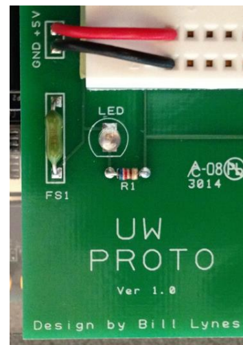
Figure 5: Fuse and blue LED (unlit) found in a corner of the UW prototyping board.
