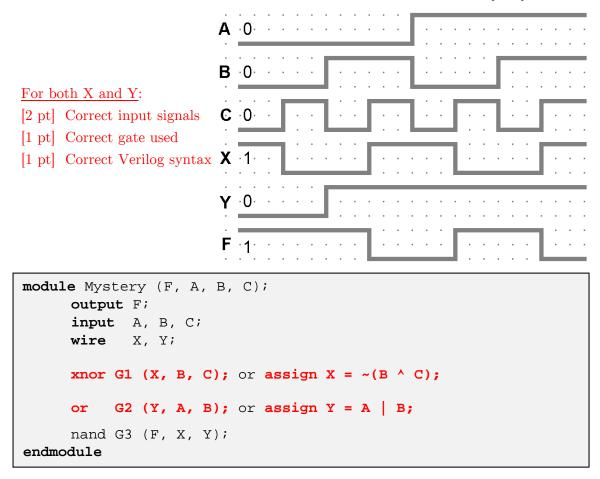
(B) The snippet below is from a Verilog testbench. Draw out the waveforms. [4 pts]
