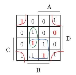
$$= \overline{B}\overline{D} + BC + \overline{A}BD$$
