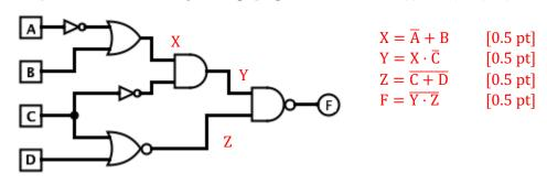
(B) Find a minimal implementation of the function below using only **2-input NAND gates**. *We will only accept circuit diagrams.* [6 pts]
